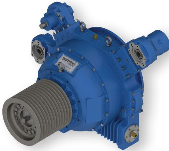
Mounted between the power take-off and the engine, the WPT® Power Pump Drive (PPD) is a rugged and versatile unit providing for multiple live or clutched pumps. As the PPD is self-contained, no external lubrication is required. Flexible couplings on the input side dampen torsional vibrations and are standard on all WPT PPDs.
